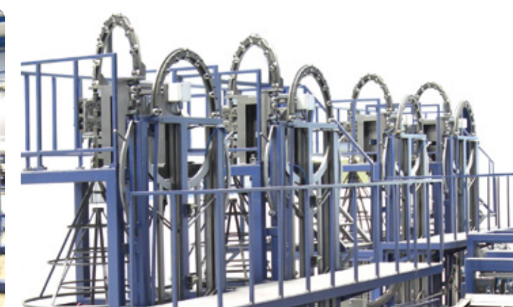
Overhead De-Coiling Stations for up to 8mm 3T Coils, with Incorporated Loop
