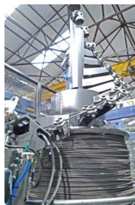
Patented Overhead De-Coiling Station for up to 12mm 6T Coils
