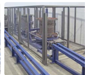
De-Coiling Stations for up to 3T Vertical Spools
