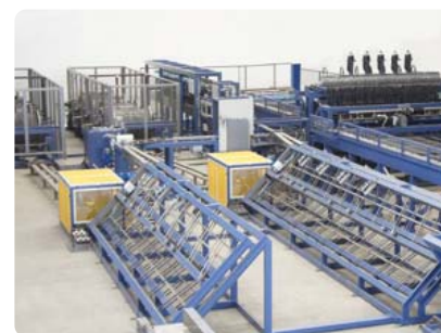
De-Coiling Stations for up to 3T Horizontal Spools, with Loop Accumulators
