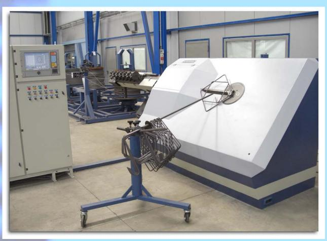
50% higher production output, compared to conventional benders, due to retractable bending pin and cutting without reversing.
