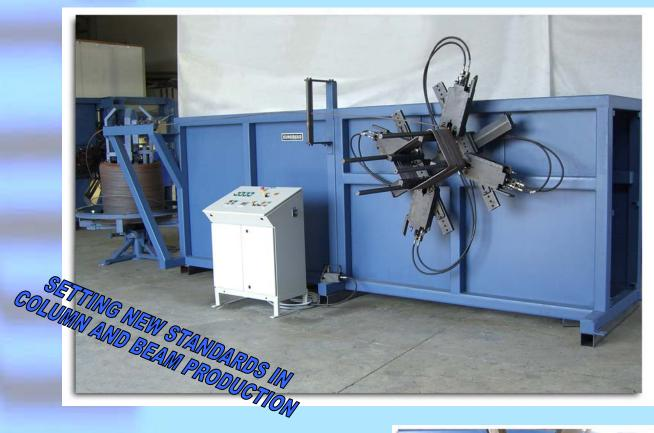
The SPIRAL SP series of spiral benders have been developed for the high-speed production of precision square/rectangular shaped spirals (PATENTED).
