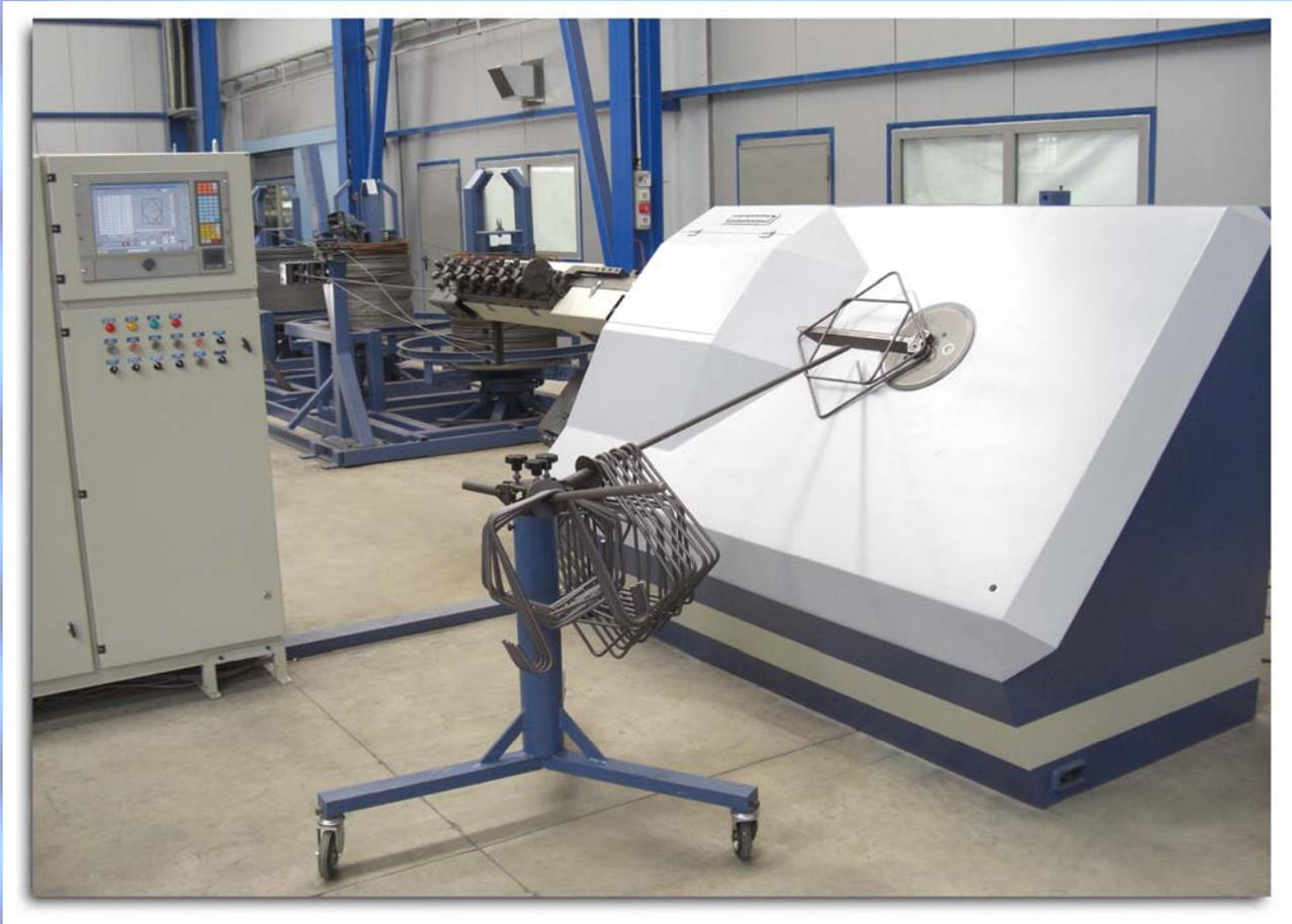
***50% higher production output, compared to conventional benders, due to retractable bending pin and cutting without reversing.***
